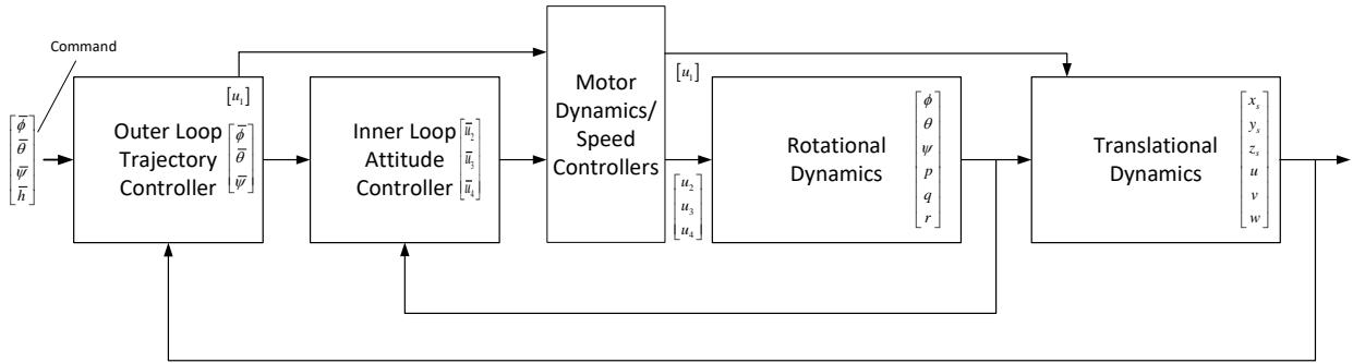
In this project, we will focus on the hover (altitude/rotational) control system. Altitude is  $h = z_s$ .
